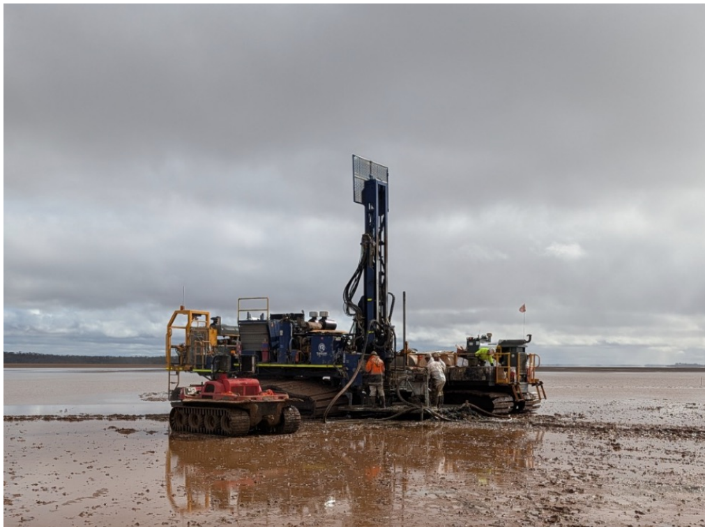
Picture – Aircore drilling underway on Lake Cowan.
