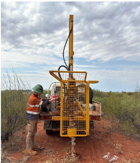
Magnetotelluric (MT) Crew deploying station; augur drill for vertical probe.
